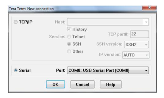
Left-click the "Serial" radio button and use the drop-down "Port" control to select the proper COM port for your NinoTNC. Left-click the OK button to continue.
