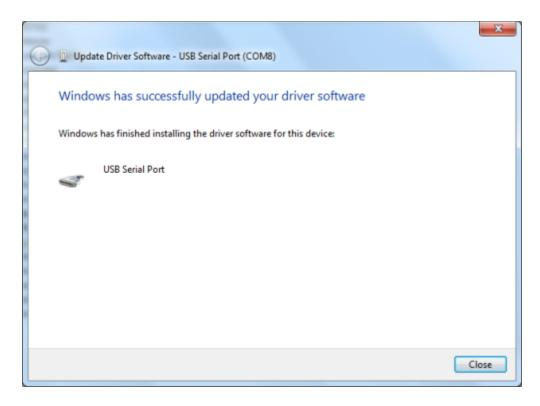
An "Installing Driver Software" window will briefly appear followed by a new window which should indicate the successful installation of the driver software. This window also indicates the COM port assigned to the new "USB Serial Port" device in the top line (COM8 in this case). Left-click the "Close" button.
