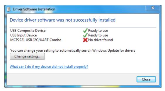
Note that while drivers for a "USB Composite Device" and "USB Input Device" were successfully installed, no device driver was installed for the "MCP2221 USB-I2C/UART Combo" ("No driver found").
