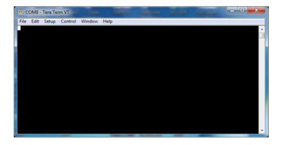
Use the "Setup" tab to select the "Serial Port" settings. Make sure the serial port values match the settings you used in Device Manager and the following image (your COM port will likely differ).
