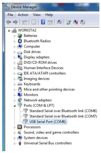
Now that the Microchip driver has been installed, it is necessary to configure the serial port for communication with the NinoTNC. Right-click the "USB Serial Port (COMx)" entry and select "Properties". The "Properties" window will appear.
