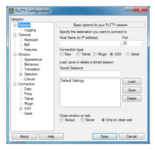
Note that "SSH" is the selected "Connection type", but you need to use the "Serial" type, so left-click the "Serial" radio button. The correct "Serial line" and "Speed" should now appear above the "Connection type" radio buttons.
