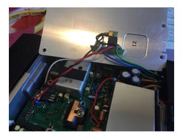
Unsolder red, black, white. Cut green and blue at add-on map module. Remove module. Then
